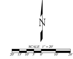
BASIS OF BEARINGS - BEARINGS ARE BASED ON STATIC GPS OBSERVATIONS. REDUCED USING DATUM - HORIZONTAL NAD 83, VERTICAL NAVD
